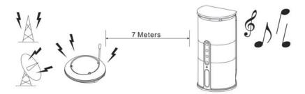
Your speakers are now portable and can be carried freely from room to room, without disruption. Should you encounter any sound distortion (signal cuts off or carries distortion), press the speaker's "AUTO TUNE" button to maximize the best reception.
